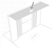
**Step 2** Attach the counter to the bracket and secure it in place.
