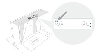
**Step 4** (Optional) Tilt the counter to the desired angle by turning the Screws B (Red) located next to the counter.
