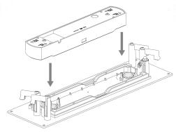
**Step 3** Clamp the bracket with the attached counter onto the ceiling and secure it by fastening 4x Screw A (Blue). Additional breakable holes are provided on each corner for direct mounting.
