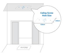
**Step 3** Attach butterfly bracket and mount the drop pole onto the ceiling with 4x screws.
