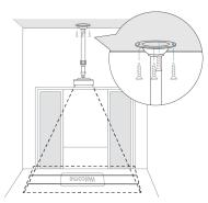
Step 4 Connect the Cat5 cable through the tubes of the drop pole.  $\ensuremath{/\!/}$
