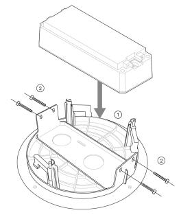
**Step 3** Clamp the bracket with the attached counter onto the ceiling and secure it by fastening 3x Screw A (Blue). Additional breakable holes are provided on each corner for direct mounting.
