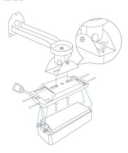
**Step 3** Mount the bracket on the wall with 2x screws and wall plugs.
