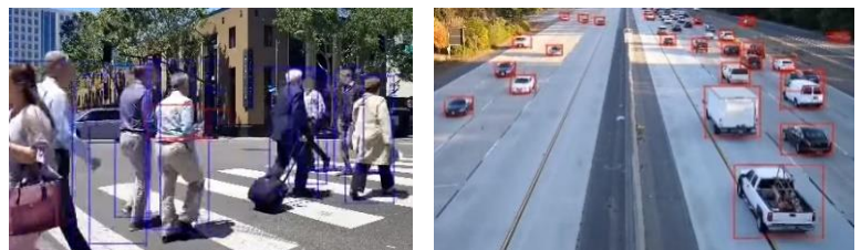
Figure 2: Screenshots from video of Centroid performing object detection on four 1080p30 streams running at a throughput of 500 megapixels per second (MP/s).
